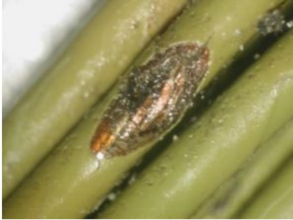
*Figure 1 Breached F-16 Kapton Wire*
