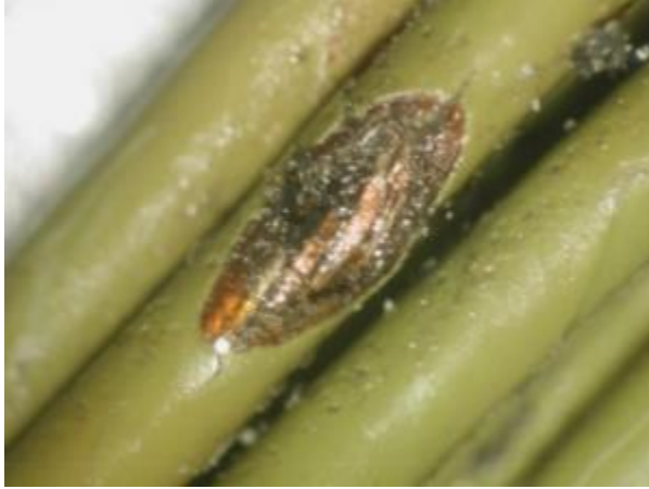
Figure 1 Breached F-16 Kapton Wire
