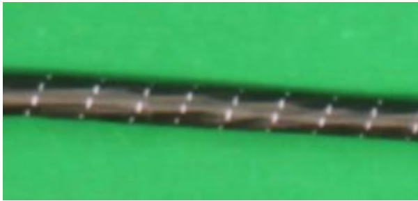
Figure 4 Non-Flight Control F-16 Wiring Harness
