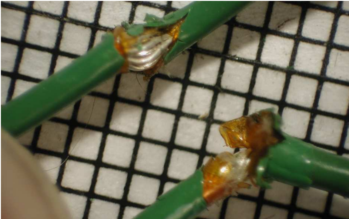
Figure C-6: Photo: H16DW651-wires 54 and 55. Background grid is 1mm long by 1mm wide. Wires 54(top) and 55(bottom) as seen under a microscope. Conductor Exposed.
